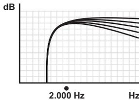
By increasing the resistance R, the amplitude will be reduced in the super-high frequency range. Remark: The bigger the value of R, the smaller the amplitude.
