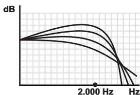
As for increase inductivity, the amplitude within the higher range is reduced. If the amplitude on the cut-off range is too quiet, the amplitude can also be reduced by reducing inductivity. Notice that on variation of inductivity, the characteristic of the filter will change.
