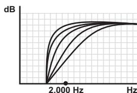
As for reduced C capacitance, the amplitude within the lower range is reduced. If the amplitude on the cut-off range is too quiet, the amplitude can also be increased by increasing C. Notice that on variation of capacitance, the characteristic of the filter will change. By large capacitance, the power which is supplied to the tweeter, strongly increases.
