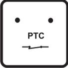
The crossover offers also the possibility to bridge the PTC (tweeter protection circuit) (Section 1). This operation brings minimal acoustic advantages, however the tweeter is not protected against overloads. Also this setting is reserved for specialists, who know the advantages and drive the system with the right power. The "6dB" setting is absolutely dangerous for the tweeter!
