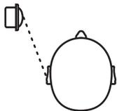
If tweeters are installed by "indirect radiation" (big angle default), there are generally too much of these frequencies. The crossover can adjust the amplitude on that band.
